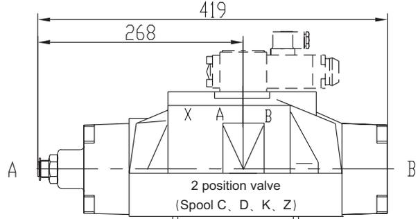
Stroke limiter on side A of valve
