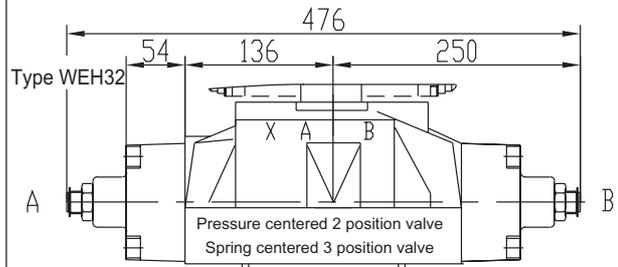
Stroke limiter on sides A and B end of main valve
