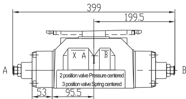
Stroke limiter on sides A and B end of main valve
