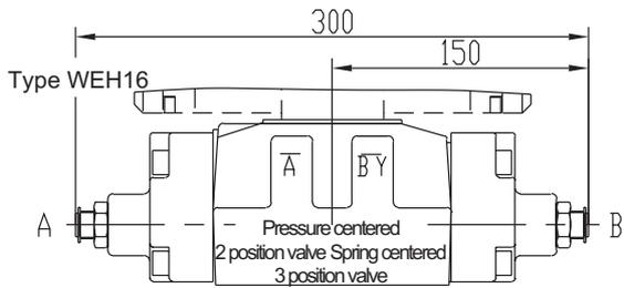
Stroke limiter on sides A and B end of main valve
