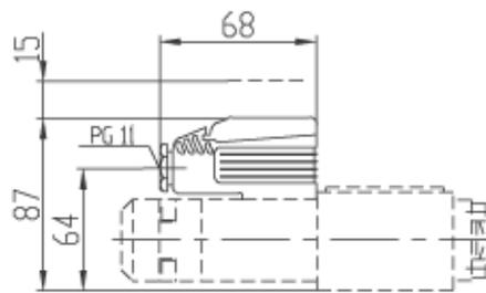
**Additional equipment : The stroke limiter**
